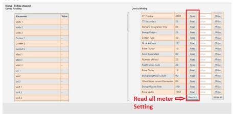
• If users want to change any parameter value Like CT, PT Ratio etc. enter value in "New Value" column w. r. t. parameter and click "Write" button.
