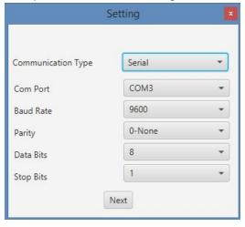
**Please Note**- Selected Baud Rate, Parity, Data Bits, Stop Bits setting must be the same as in the actual meter of serial communication settings.
