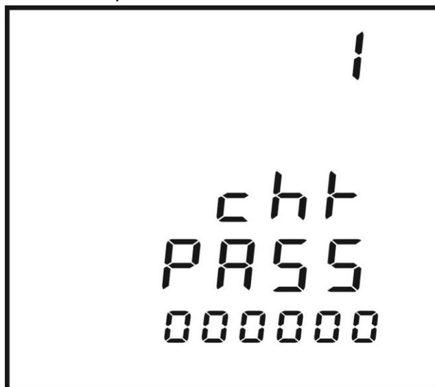
**2<sup>nd</sup> screen:** Communication address setup screen can setup communication address. Range is 0 to 255 any integral numbers (exceed 255, unpredictable).
