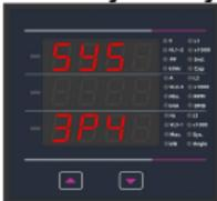
This screen is used to set the System Type 3P4W, 3P3W, 1P3W & 1P2W.
