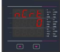
This screen allows the user to set Low noise current cutoff in mA. Pressing "⬆" key advances to the Demand Integration Time.
