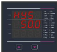
This screen allows the user to set Hysteresis for relay output. The allowable range is 0.5% to 50 % of Trip point. Enter value, prompt for first digit. (Blinking digit denotes that value will be changing
