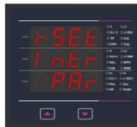
Reset option “Intr” select: (Reset Number of Interrupt) Pressing “ $\downarrow$ ” key will select the value and will reset number of auxiliary supply interruption count.
