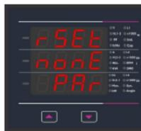
Reset “None” select: Pressing “ $\downarrow$ ” key advances to Reset Parameter selection screen (See Section 3.2.3). Pressing the “ $\uparrow$ ” key will enter the Reset option mode & scroll through parameter and wrapping back to none.
