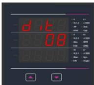
This screen is used to set the period over which current and power readings are to be integrated. The unit of displayed readings is minutes.
