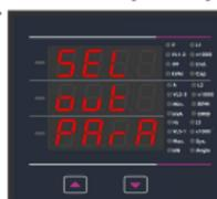
This screen will allow the user to select output option like "Relay" Output.
