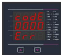
The meter has not accepted the password entered. Pressing the "⏏" key will return to the enter password stage. Pressing the "⏏" key exits the password menu &
