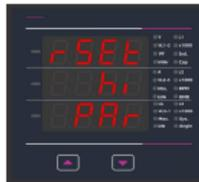
Reset option “hi” select: (Reset Max parameters) Pressing “ $\downarrow$ ” key will select the value and resets all Max parameters.
