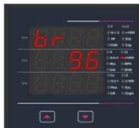
This screen allows the user to set Baud Rate of RS 485 port. The values displayed on screen are in kbaud. Pressing "←" key advance to the Party Selection screen (See Section 3.2.2.3).
