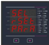
This screen is used to reset the different parameters. Pressing the "⏪" key allows the user to reset different system parameters (See Section 3.2.3.1). Pressing the "⏪" key
