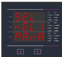
This screen applies to the Relay Output option selection. Pressing "↵" key will select the rEL1 Output Selection Screen (See Section 3.2.4.1.1). Pressing the "⇐" key will advance to the Quit screen.
