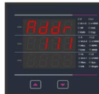
Enter Address for third digit. Press the "→" key to advance to next Screen "RS485 Baud Rate" (See Section 3.2.2.2). Pressing the "←" key will re-enter the Address edit mode.
