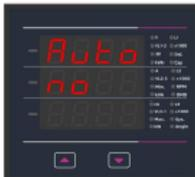
This screen allows user to enable screen scrolling. Pressing "⬆" key advance to the No. of Poles Selection screen (See Section 3.2.1.9).
