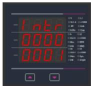
This screen displays the total no. of times the auxiliary supply was interrupted. Even if the auxiliary supply is interrupted count will be maintained in internal memory. To reset No of Interruption manually see Section
