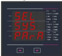
This screen is used to select the different system parameter like "System Type", "CT Ratio", "PT Ratio", pressing the "⏪" key allows the user to set different system parameters (See Section 3.2.1.1 to 3.2.1.7).
