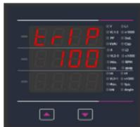
The allowable range for High Alarm and Low Alarm can be referred from table 2. Enter value, prompt for first digit. (Blinking digit denotes that value will be changing).
