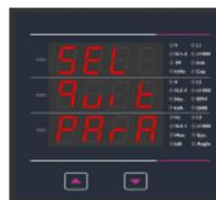
This screen allows the user to quit the output option. Pressing "↵" key will advance to the Output Parameter selection (See section 3.2.4). Pressing the "⇐" key will go back to Relay output option (See section 3.2.4.1).
