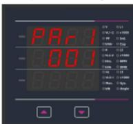
Pressing "⇐" key advance to the Limit Configuration Selection screen (See Section 3.2.4.1.1.1.2). Pressing the "↵" key will enter the Limit Output edit mode. Pressing the "⇐" scroll the values, as per Table 2: "Parameter for Limit Output".
