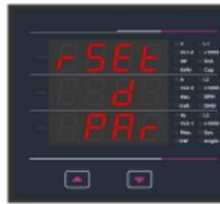
Reset option “d” select: (Reset Max Demand parameters) Pressing “ $\downarrow$ ” key will select the value and resets all Max Demand parameters.
