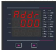
This screen applies to the RS 485 output only. This screen allows the user to set RS 485 parameter for instruments.
