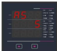
This screen is used to set the value for Current Transformer Secondary value, "5" for 5A or "1" for 1A can be selected. Pressing "⬆" key advances to the Demand Integration Time (See Section 3.2.1.6).
