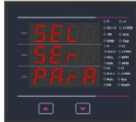
This screen is used to select the different communication parameters like "Address", "RS485 Parity" and "RS485 Baudrate". Pressing the "⏪" key allows the user to set different communication parameters.
