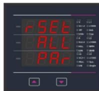
Reset option “All” select: (Resets ALL resettable parameter) Pressing “ $\downarrow$ ” key will select the value and advance to the reset ALL parameters.
