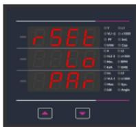
Reset option “Lo” select: (Reset Min parameters). Pressing “ $\downarrow$ ” key will select the value and advance to the reset all Low parameters.
