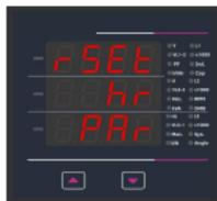
Reset option “hr” select: (Reset ON Hour & Run Hour). Pressing “ $\downarrow$ ” key will select the value and will reset On hour & Run Hour.
