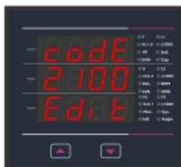
New/Change Password, first digit entered, prompting for second digit. (Blinking digit denotes that value will be changing). Pressing the "⏏" key will scroll the value of the second digit from 0 through to 9, the value will wrap from 9 round to 0.
