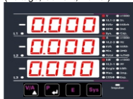
Screen 1 : System Values (Voltage, Current, Power)
