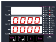
Screen 4 : Reactive Energy (Capacitive)
