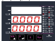
Screen 2 : System Values (Frequency, PF)
